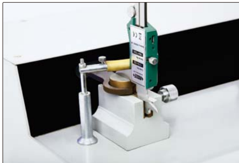
lapping measuring surfaces of caliper lower jaws
