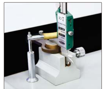
lapping measuring surfaces of caliper lower jaws
