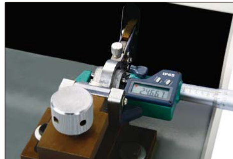
lapping measuring surfaces of outside micrometer
