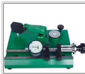
inspect accuracy of dial indicators (range 0-25mm)
