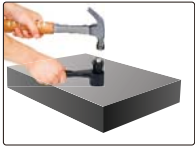
hammer impact to apply test force
