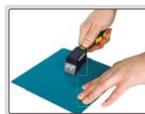
step 1: make grid cutting on surface
